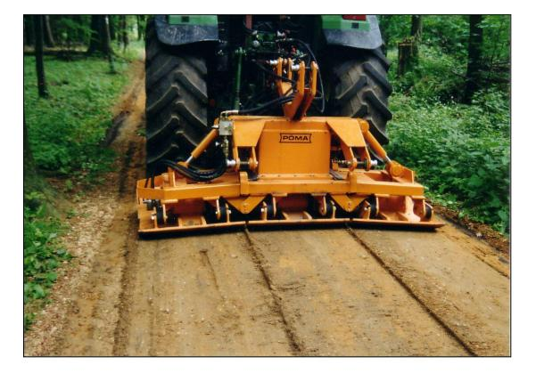
The PÖMA – RP240 is developed for compacting and smoothing of reconditioned gravel roads and for landscaping. The high impact force makes a very good job for compacting.
